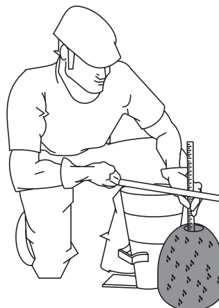
Figure 60-F. Slump Test (Measurement)
